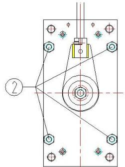
3. The braking test again, check whether single arm brake, failed to system still need to install the step 2 again, until can one-armed brake;
